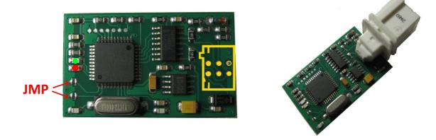
**NOTE:** emulator is not reusable – it permanently locks to car after about 15 successful startups. Although you can test it on various cars while test counter do not exceed this limit - every new car resets counter back to 0 and alignment procedure starts once again (first startup).
