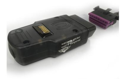
2. Connect the device to the diagnostic plug
