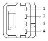
pin1: not used (no wire), pin2: +PWR (switched), pin3: GND, pin4: LIN.
